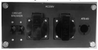
Overload is forbidden in case of single phase receptacle output.
