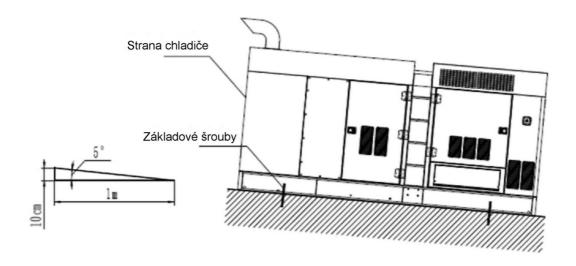
If the ground or floor may be wet from time to time, the foundation should be raised off the floor. This will ensure dry ground for the generator and its operator. It also minimizes corrosive action on the base frame.
