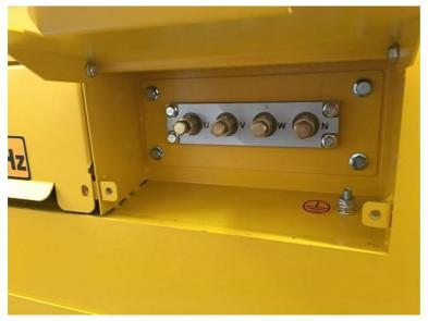
Connect the cable to the three-phase and four-wire terminals listed above.
