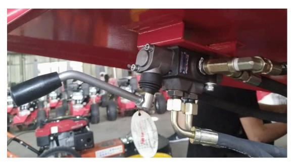
By operating the handle, there are 3 functions of the feeding roller: Feeding, Reversing, hold-on.
