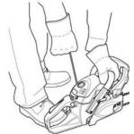
8. While holding the saw unit securely on the ground, pull the starter rope vigorously.
