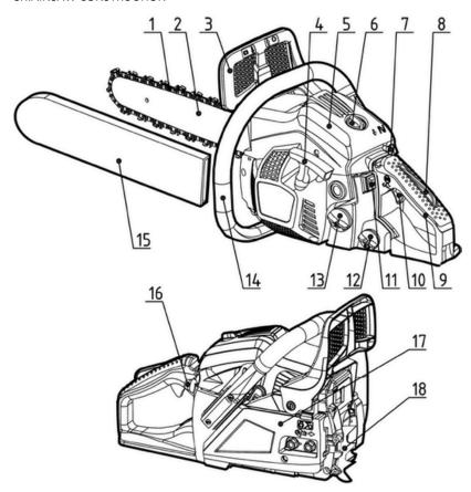
1.Saw chain 2.Guide bar 3.Front hand guard 4.Starter handle 5.Air filter cover 6.Lock nut
