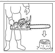
2) Holding the chain saw horizontally, release your hand from the front handle, hit the tip of the guide bar to a stump or a piece of wood, and confirm brake operation. Operating level varies by bar size. In case the brake is not effective, ask our dealer inspection and repairing.
