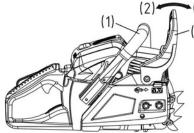
(4) Normally, the brake is activated automatically by (4) inertial force. It can also be activated manually by pushing the brake lever (Front handle guard) down toward the front.
