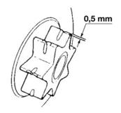
**4. Sprocket** Check for cracks and for excessive wear interfering with the chain drive. If the wear is considerable, replace it with new one. Never fit a new chain on a worn sprocket, or a worn chain on a new sprocket.
