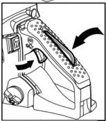
9. When firing occur, press the throttle trigger to allow the choke return to the running position and pull the starter handle again to start the engine.
