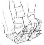
Before you start the engine, make sure the saw chain is not contacting anything. Make sure the chain brake always is activated before each starting.
