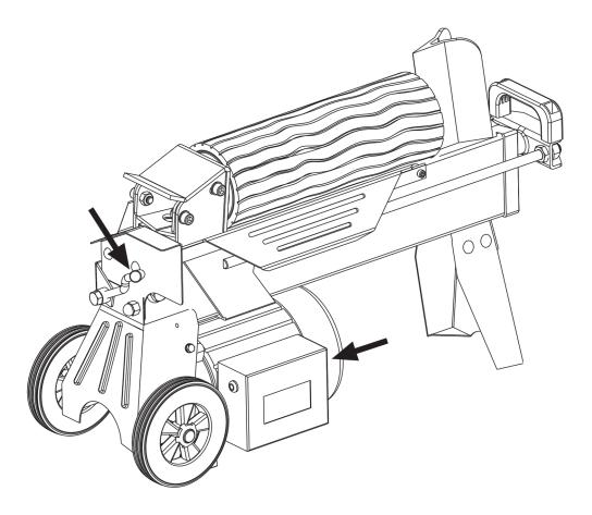
This log splitter is equipped with "ZHB" control system that requires to be operated by both hands of the user – Left hand controls the hydraulic control lever while right hand controls the pushbutton switch. The log splitter will freeze upon absence of either hand. Only after both hands release the controls, the log pusher starts to return backward to the starting position.
