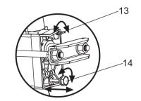
Before operating the log splitter, the Bleed Screw should be loosened by some rotations until air can go in and out of the oil tank smoothly.
