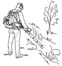
Engine speed should be adjusted to the type of material to be removed, it is seldom necessary to use full throttle, and many work procedures can be done at half throttle:
